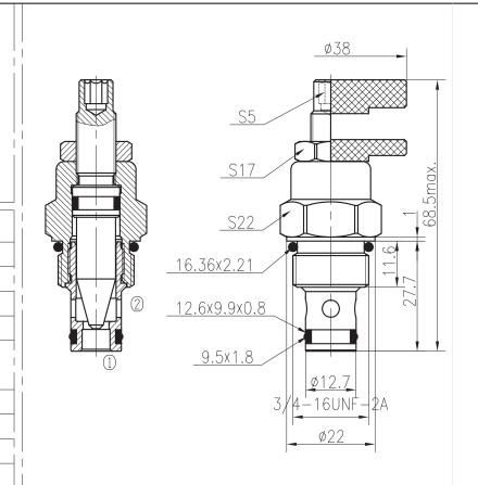
The valve reduce its orifice value from fully opened to fully close with clock—wise adjustment rotation.
