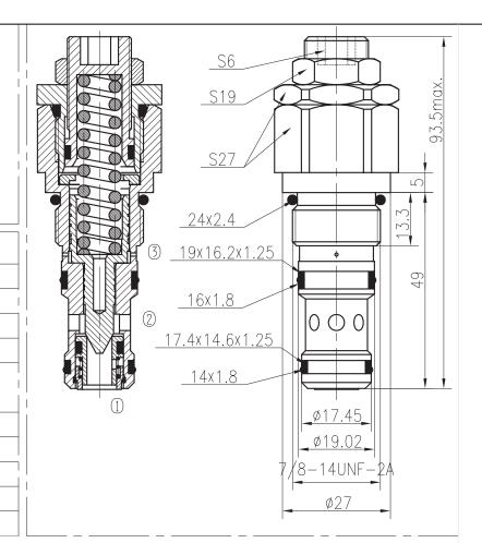
The valve controls moving load and preventing it from running ahead of the pump,locking the load in any position,it also provides static overload and thermal enpansion protection.
