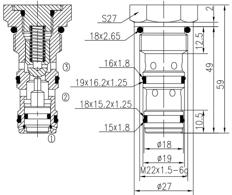
The valve allows flow from ② to ③ with very low pressure drop, while blocks flow from ③ to ②.
