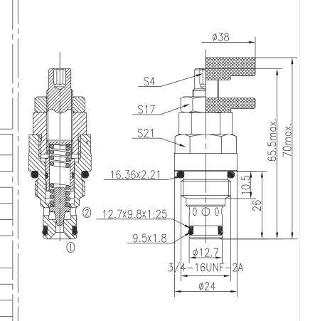
The valve blocks flow from 0 to 0 until 85% pressure is present at 0. With the continued increase pressure on 0,0 to 0 began to overflow, until to the spring's maximum pressure.
